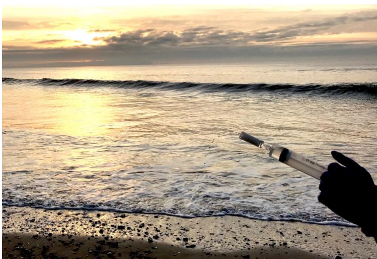
Sterivex filter being used to collect environmental DNA from seawater
