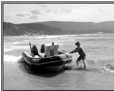
Above:- "Banga", a 5.5-metre Gemini semi-rigid rubber duck, is suitable to launch in most surf conditions along the South African coast. (Picture © Dr Angus Paterson)
