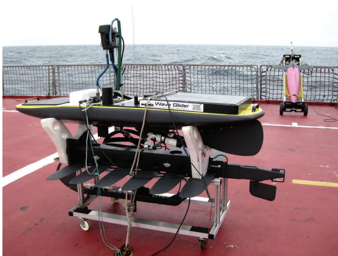
Wave Glider (front) and Seaglider (back) before deployment into the Southern Ocean. The experiment lasted 4.5 months where both gliders collected a suite of high resolution variables.
