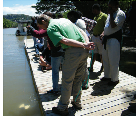
Participants using a Secchi disc to estimate the penetration of light into the Kwelera Estuary (Photo: G Snow).
