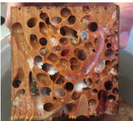
A block of wood bored by a shallow-water, wood-boring clam species.
