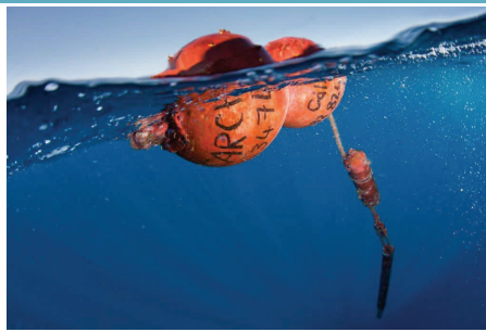
A retrieved ATAP receiver and acoustic release. Photo by Ryan Daly.
