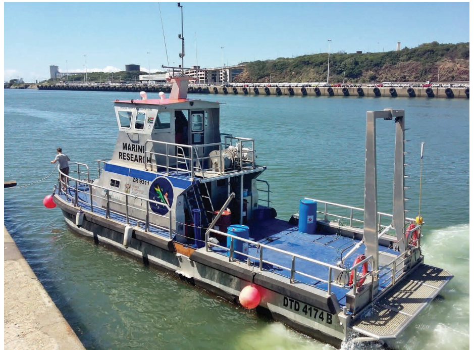
Powered by jet-propulsion engines, R/V Phakisa will enable research in strong current conditions. Photo – Ryan Palmer © NRF-SAIAB.
